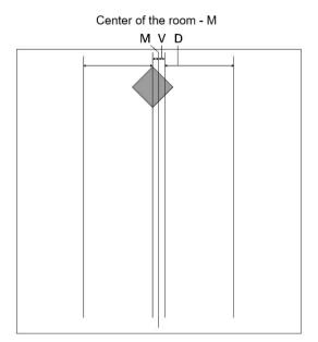
Now you need a square elastic flooring tile (this must be exact) as a laying aid to be able to lay the planks easily. This is placed with the opposite tips on one of the two displacement dimension lines and temporarily fixed using double-sided adhesive tape.
