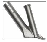
Set the welding machine to approx. 450°C. Use a 5.0mm speed welding nozzle to insert the fusion wire.
